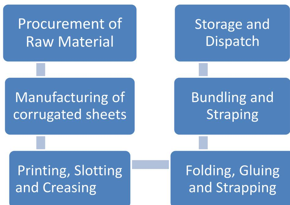
Our manufacturing process starts with procurement of raw materials i.e. Kraft Paper, adhesive for Ply bonding, adhesive for glue tab and water based ink. Kraft Paper is arranged from paper mills in the form of reels as per the requirement of customer based on the GSM requirement of carton. Adhesive for ply bonding is manufactured in our manufacturing facility which uses a controlled input of native
